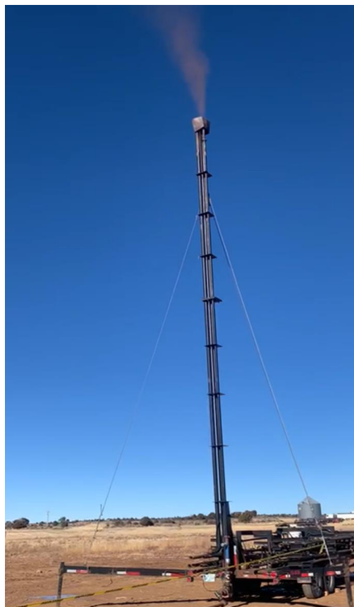
Figure 1: Jesse-1A flare stack venting reservoir helium to surface https://grandgulfenergy.com/jesse-1a-flows-helium-to-surface/
